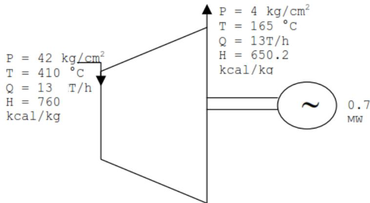
Find the cogeneration efficiency based on mentioned figure. P,T,Q and H represent pressure, temperature, mass flow rate and specific enthalpy respectively.
